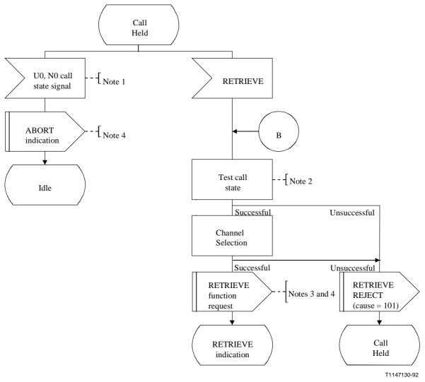
NOTE 1 – Any basic call signal which causes a transition to U0, N0 Idle shall generate this signal.
