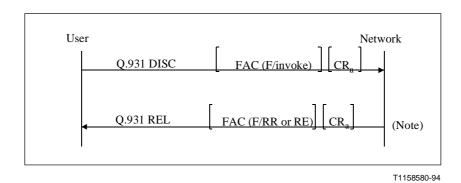
NOTE-Assume the signalling association,  $CR_a$  can be cleared together with the connection for the invoked supplementary service, otherwise a FACILITY message may be used instead.
