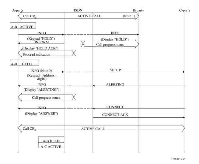
NOTE 1 - The first call is established using the normal call establishment procedures specified in Recommendation Q.931.
