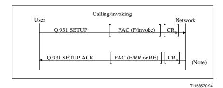
NOTE – Depending on the invoked supplementary service and the basic call control procedure, one of Q.931 messages in the network-to-user direction may be used to carry return result, return error or reject indication or even an invoke for further information.
