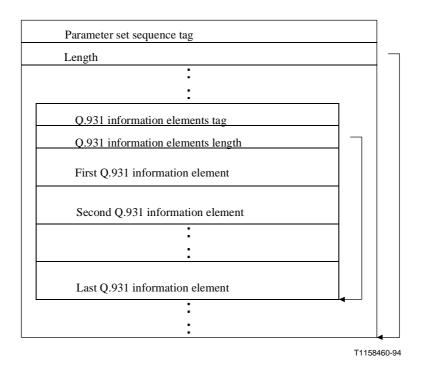
Figure 8-4/Q.932 – Encapsulation of Q.931 information elements
