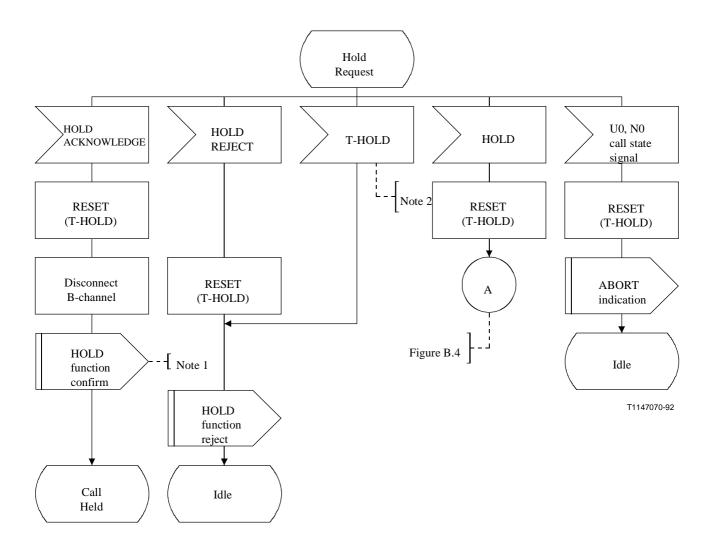
$NOTE\ 1-This\ signal\ is\ sent/received\ to/from\ the\ appropriate\ supplementary\ service\ entity\ using\ the\ HOLD/RETRIEVE\ functions.$
